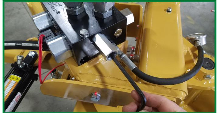
*Remove relief cap and insert Allen wrench*
