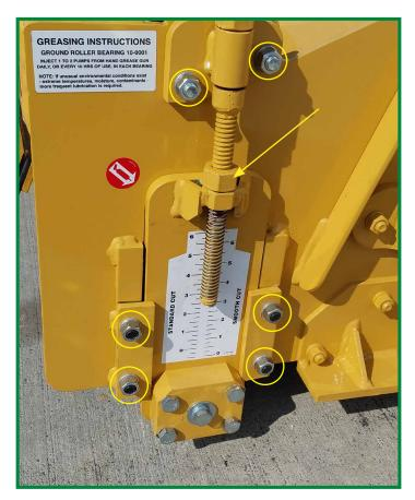
Loosen stop nut and remove bolts
