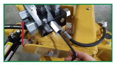
Remove relief cap and insert Allen wrench
