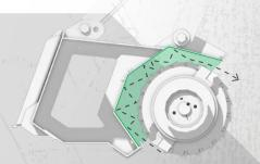
Drum shell shaped to mulch effectively with first pass
