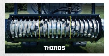
You can choose to configure your drum mulcher with TWIN MAUL™ carbide teeth on the outer edges and one of our hardened steel options in the center, as indicated above. This allows for high productivity in the center of the drum, and more durable teeth on the outside where your teeth may make more ground or rock contact. This combination optimizes productivity while minimizing your operating costs.
