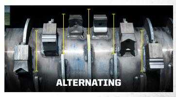
To reduce your routine maintenance, you can alternate our two hardened steel options on the drum. The **TWIN CHISEL™** is extremely easy to sharpen while still on the drum, making it quick to get ready for your next job. The **FOUR-POINT** is a more aggressive tooth, allowing you to grab and pull in material more effectively. Alternating these teeth gives you a good balance of productivity and ease of maintenance.
