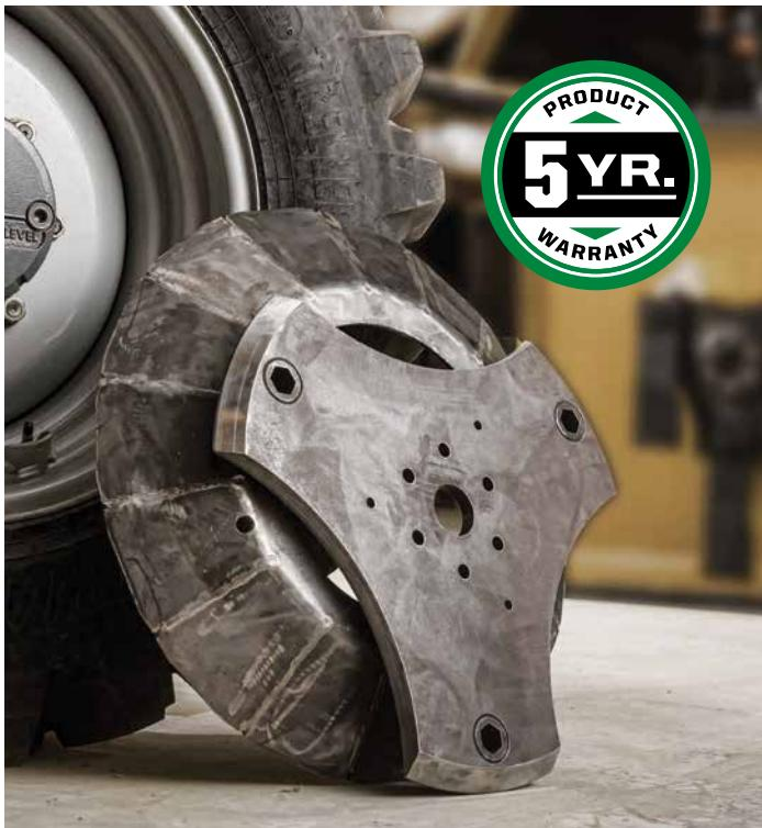
Diamond's proprietary Tri-Hex mulching disc on our rotary mowers provides greater inertia in tough conditions, and prevents material build-up between the deck and blade carrier. The disc is constructed of 1" thick 50,000 psi rated steel with hardened, replaceable inserts, giving you unparalleled durability and easy blade maintenance.
